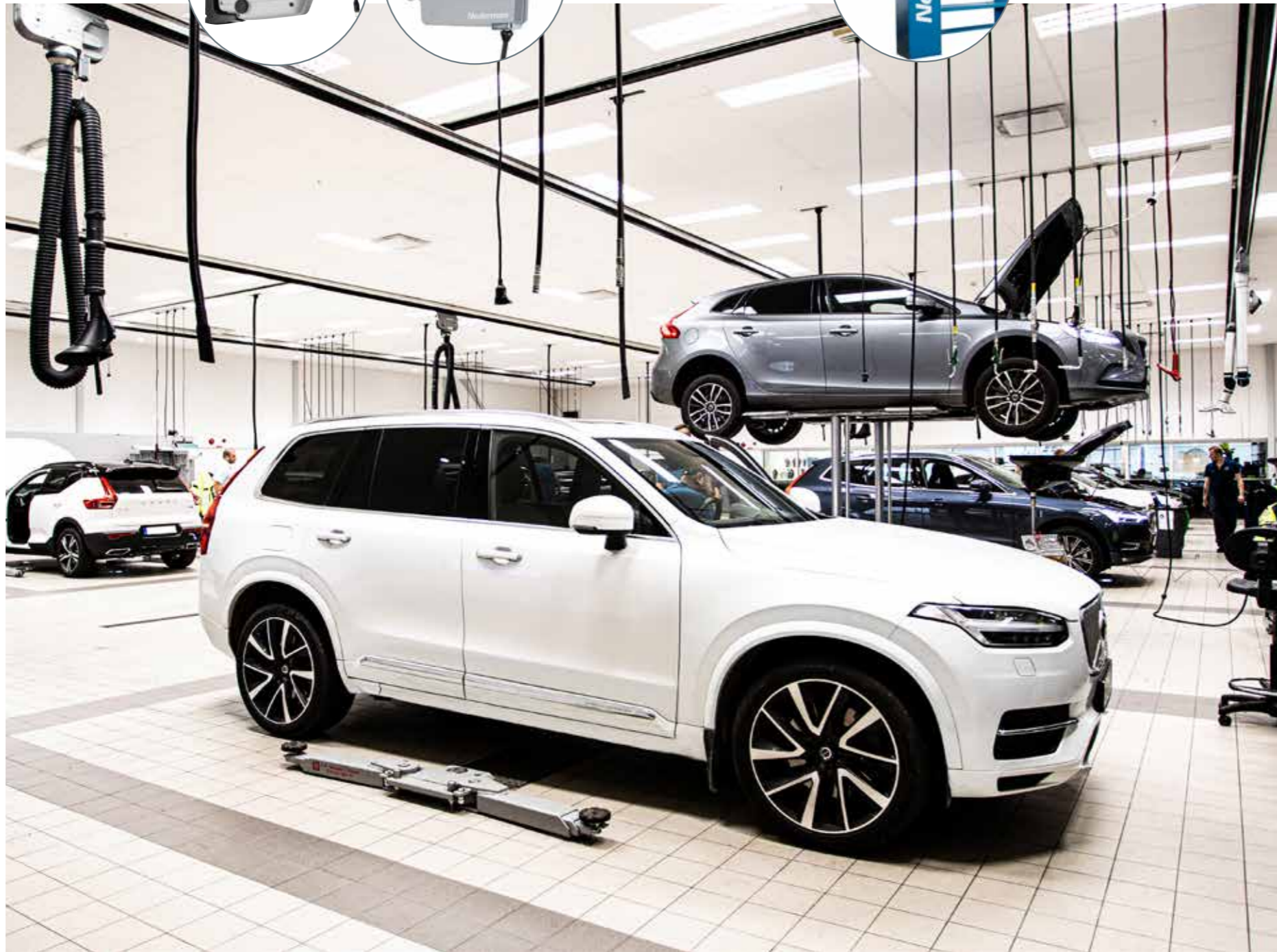
Hose reels for distributing liquids, gas and compressed air.
