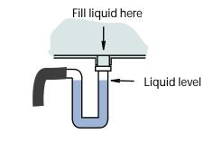
Fill the pipe with an approriate liquid, to make sure that air cannot be drawn back along the oil discharge pipe.
