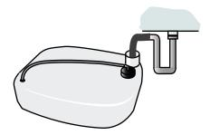
Push the container in under the filter unit, and put the hose on the pipe into the opening of the container.
