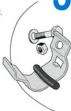
**ENGLISH** Fasten the tubular support on the fan with clamps, screws and locking nuts.
